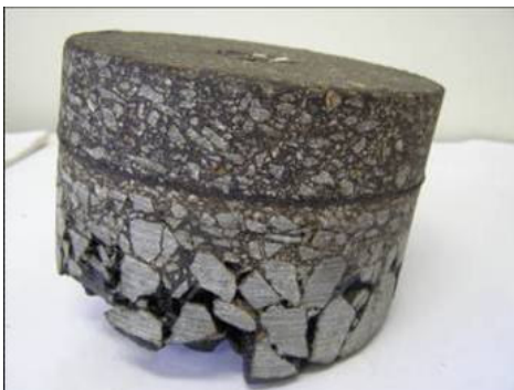
Figure 8.1: Cored sample showing effectiveness of ARI
